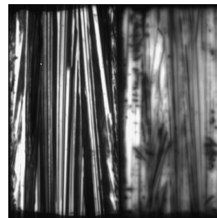
Fig.3 PL image of an n-type (left) and a p-type (right) string ribbon silicon wafer side by side.
